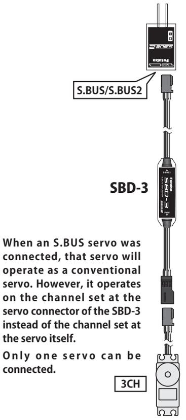
When an S.BUS servo was connected, that servo will operate as a conventional servo. However, it operates on the channel set at the servo connector of the SBD-3 instead of the channel set at the servo itself.
